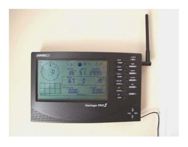
The Davis Vantage Pro 2 console receives data from the transmitter on the weather shelter. The console can receive data up to a distance of approximately 1000 feet. The above console transmits the data to Computer one which has Virtual Weather Software that uploads the data to the server, WestHost, so it can be displayed on the Glen Allen – Springfield Park website
