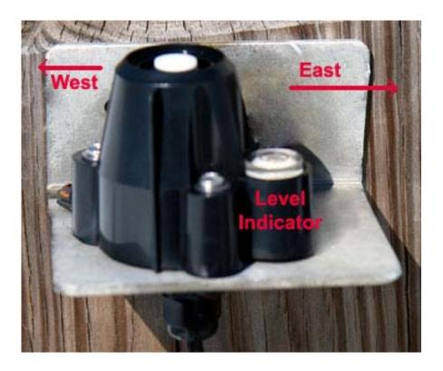
Ideally you want to place a solar sensor so you can see down to the East, South, and West horizon so the sensor receives solar radiation throughout the whole day.
