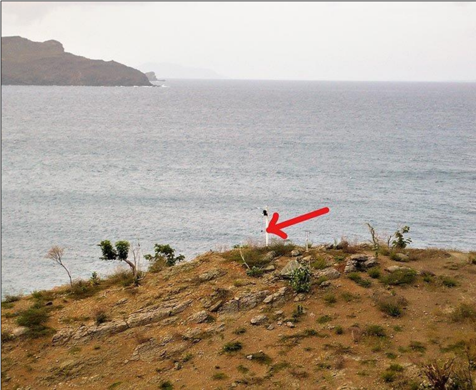
Figure 1. Serge Brin's personal weather station (PWS) on St. Barts (ISAINTBA3), after Hurricane Irma had severed the 21-foot pole housing the anemometer. The view is to the northwest from the north coast of St. Barts. Image credit: Serge Brin.
