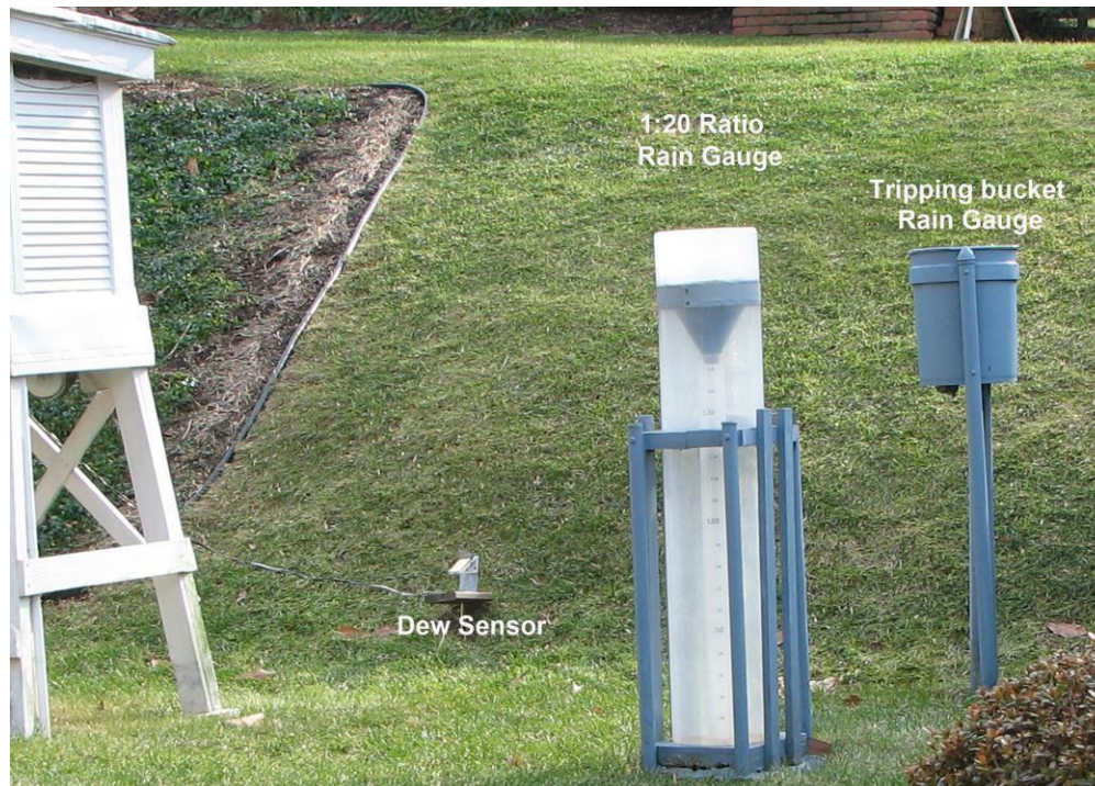
Fig. 16 A view of some of the outdoor instrumentation – The two heated tripping bucket rain gauges were located in the insulated bucket which is on the right side of the picture above.
