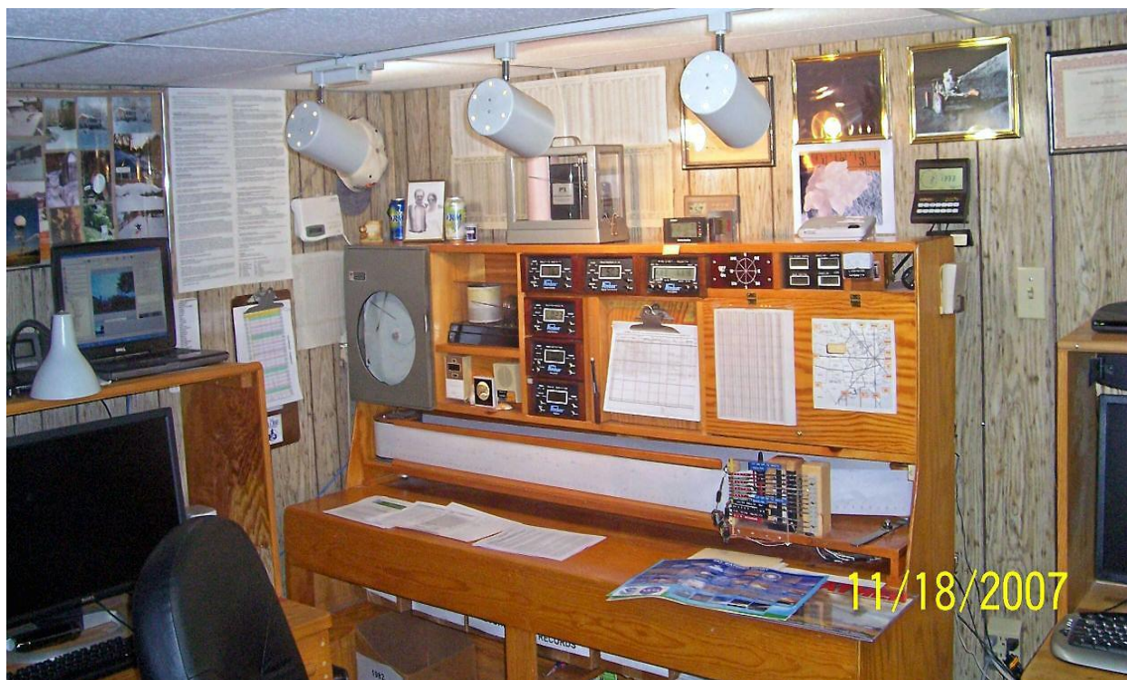
Fig. 13 This station was very complete and had backup instrumentation and even a generator to run equipment during power outages which often occurred during storms.
