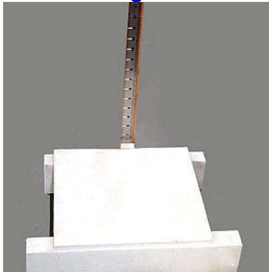
The snowboard should be painted white so that during the day it receives a smaller quantity of solar energy thus preventing melting. The measuring stick mounted to the snowboard should be divided into tenths of an inch. You should have more than one snowboard so that if an earlier snow has not yet melted before a new snowstorm impacts your area.
