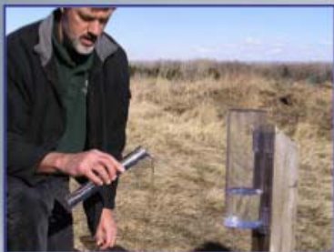
Pour out the first inch from the inner tube and write it down.
