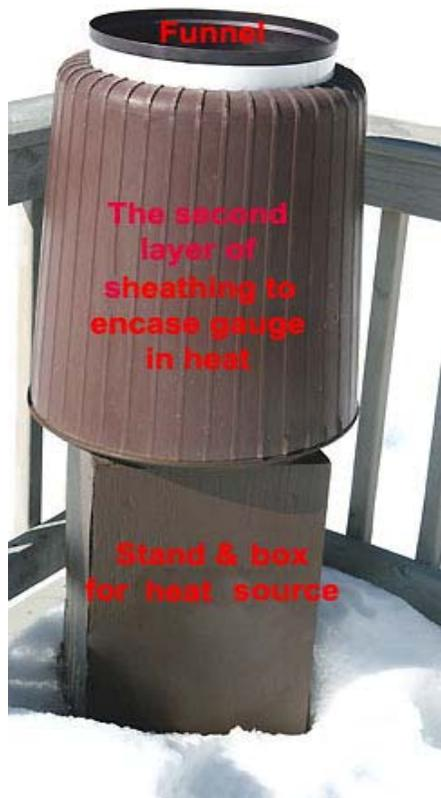
In the picture above you see the green inner cover for the 12 inch rain gauge and above you see the outer brown cover. You can see the two light sources under these two covers in the first picture. The 100 watt bulb is right below the bottom plate and the 40 watt bulb is at the edge of the cylinder. The two covers that go around the white inner cylinder are used to insulate the white cylinder and carries heat up the sides of the cylinder so no snow will build up around the top of the funnel.
