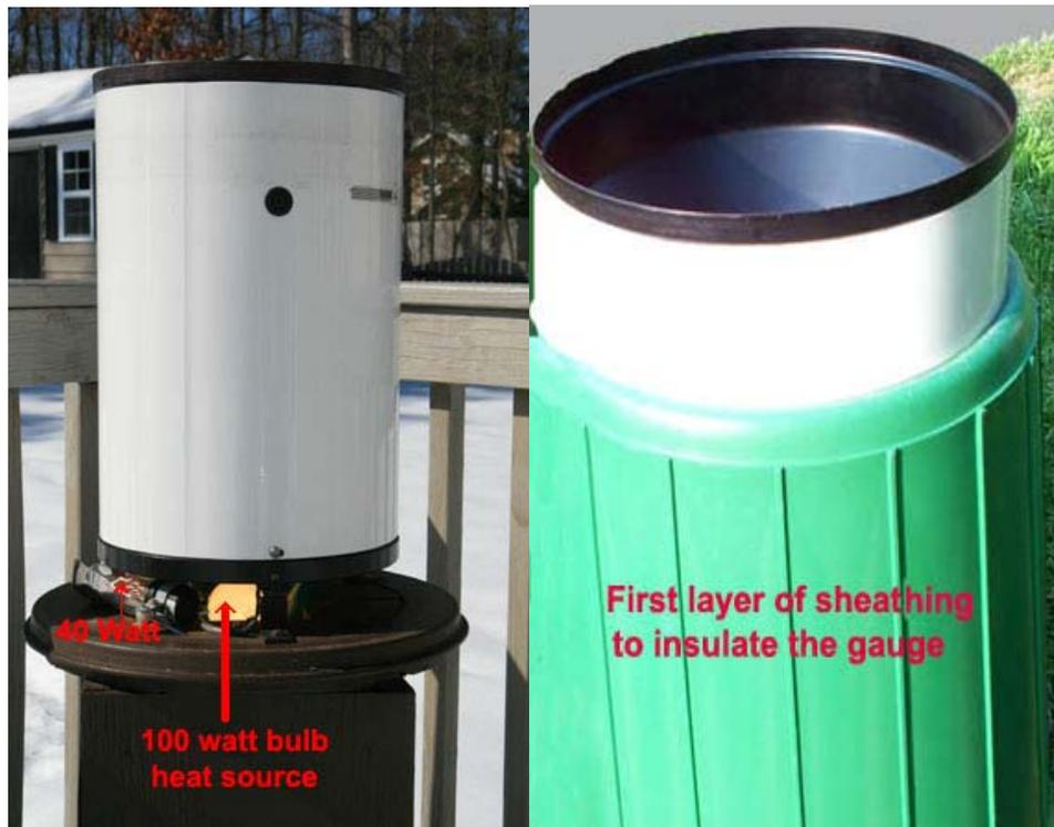
The bulb you see is the auxiliary heater; the 100 watt bulb is below the black floor plate.
