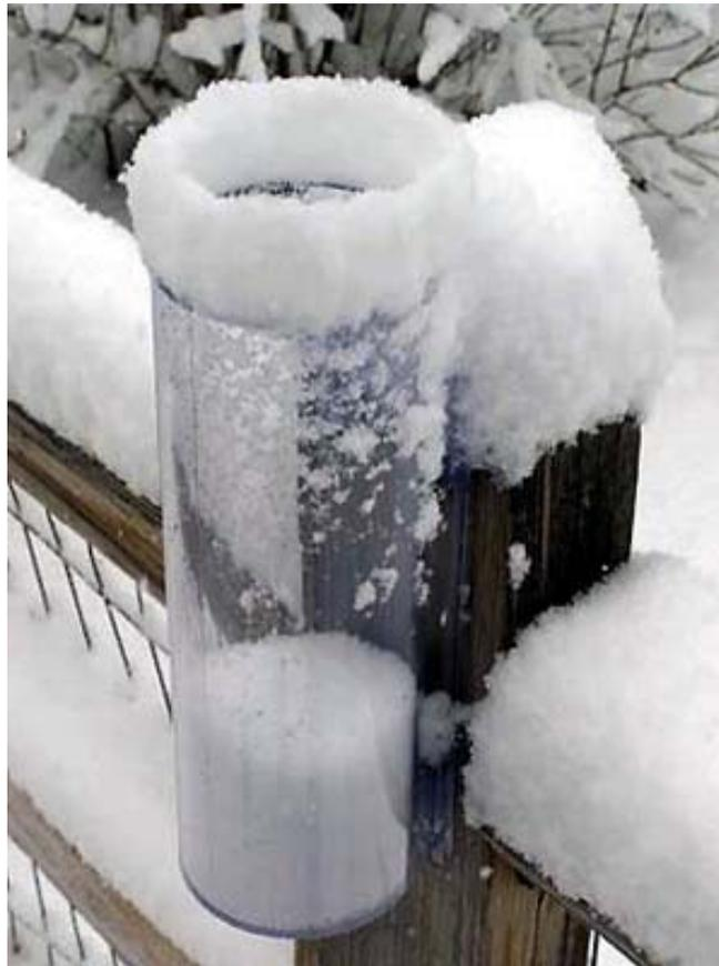
If you have a heated tripping bucket gauge and a heavy wet snow is occurring the snow will not stick to the lip of the gauge as it would to other gauges because it would melt as it fell giving greater accuracy.
