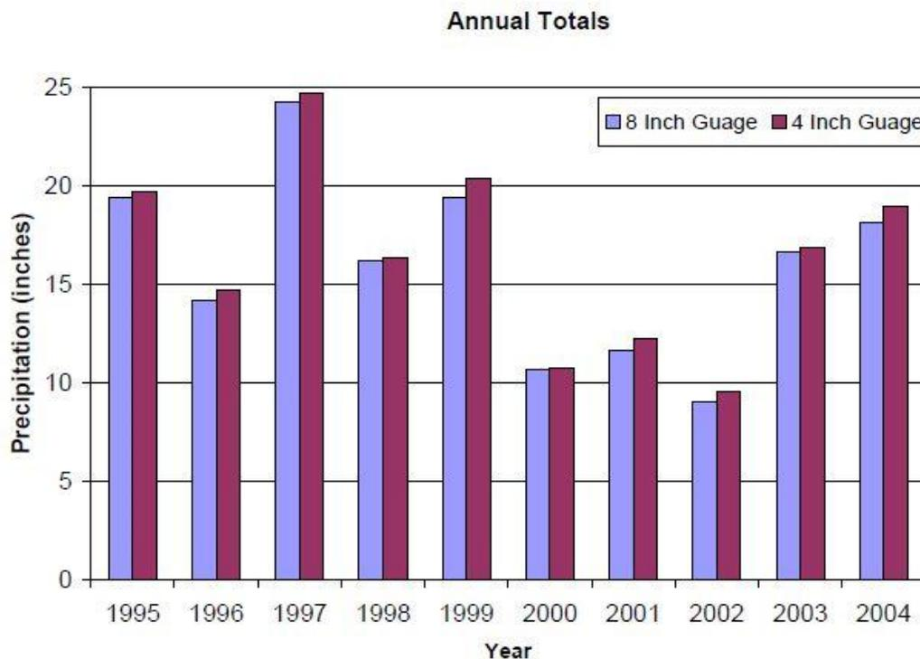
*Figure 2. Annual precipitation comparison, 1995-2004 between the 8" diameter SRG and the 4" diameter clear plastic gauge.*
